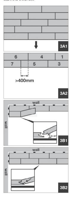
You can tap the long side of the plank into the groove by using a professional tapping block. The planks should not be joined by a single tap. To avoid damaging the planks, you must tap them together gradually.
